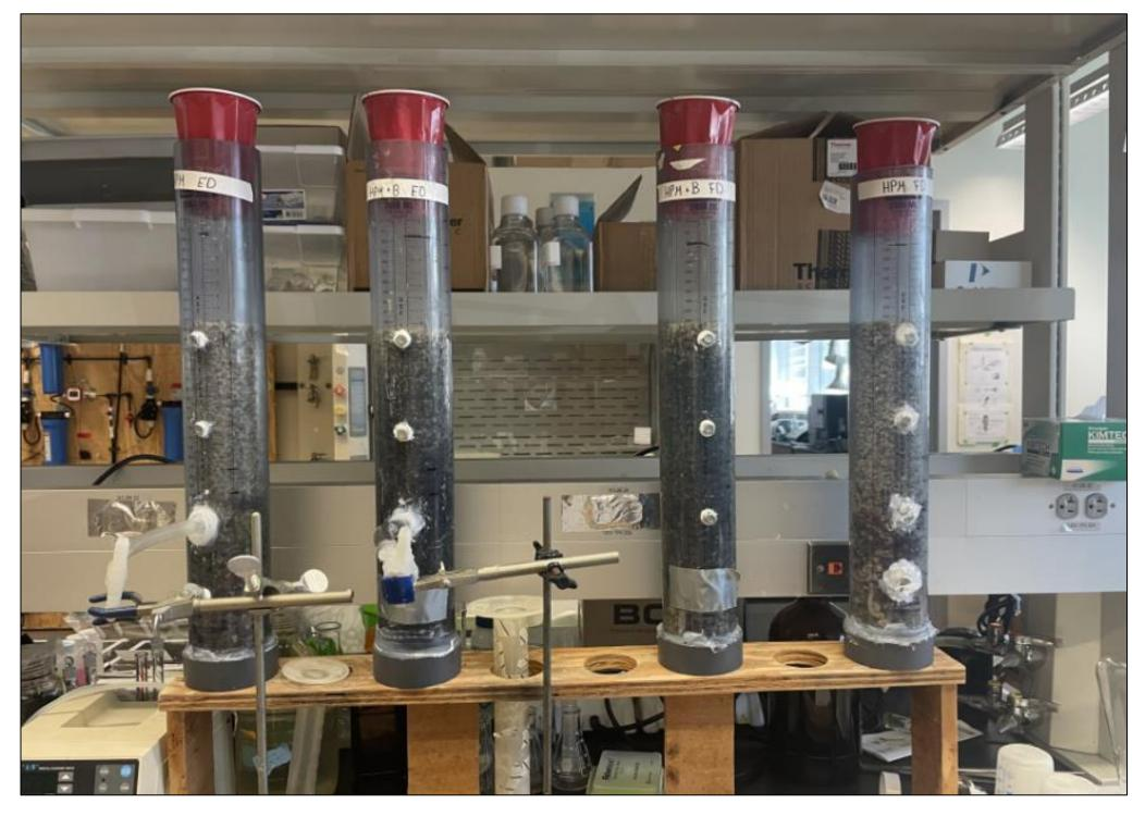
Four columns were set up to test the effect of biochar addition and outlet elevation on nitrogen removal. Determines how much of NH<sub>4</sub>+-N and NO<sub>x</sub>-N is removed through denitrification, nitrification, and adsorption with the use of biochar
