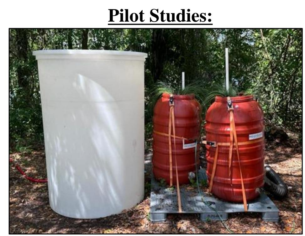
Two pilot scale systems, both with media containing biochar, were used to test the effect of outlet elevation, mulch addition and plant addition on nitrogen removal.
